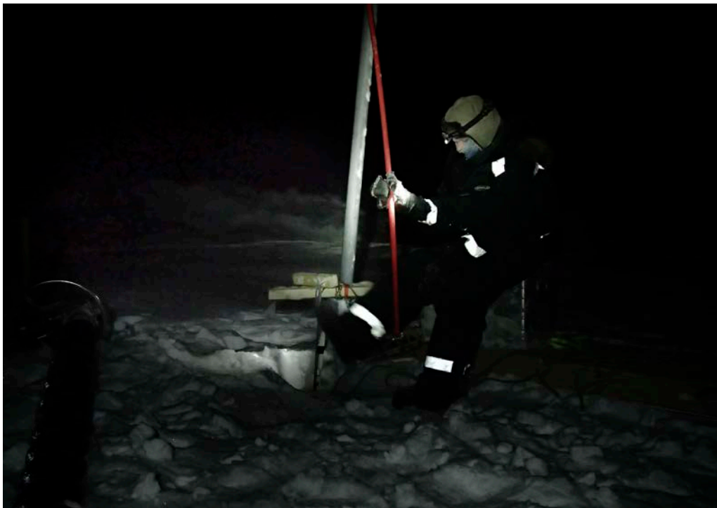
Fig. 3. Recovering the thermistor string. The supporting chain was hooked under the ice by a shackle attached to a strong rope taped to the end of the red pole. The front of the pressure ridge is barely visible in the dark background.
